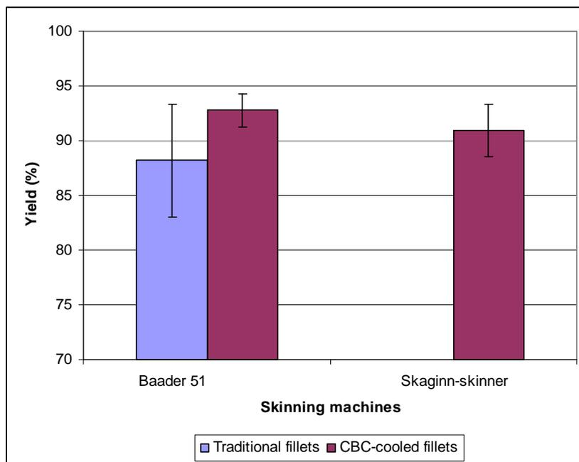
**Figure 15** The difference in yield between Baader 51 and Skaginn-skinner S3 skinning machines. Skaginn-skinner is a continuous part of the CBC-cooling process.
