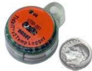
Figure 2. TidbiT v2 temperature logger used for measuring ambient air temperature.
