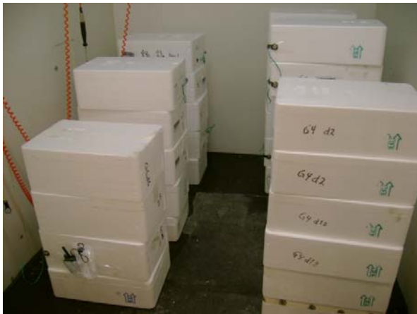
Figure 5. EPS fish box piles during storage in an air climate chamber.
