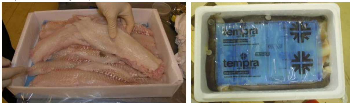
Figure 14. Fresh white fish fillets in wholesale fish boxes. Left: corrugated plastic box with no ice pack. Right: expanded polystyrene box with an ice pack on top of the fillets. Also shown are ibutton temperature loggers used for mapping product temperature.
