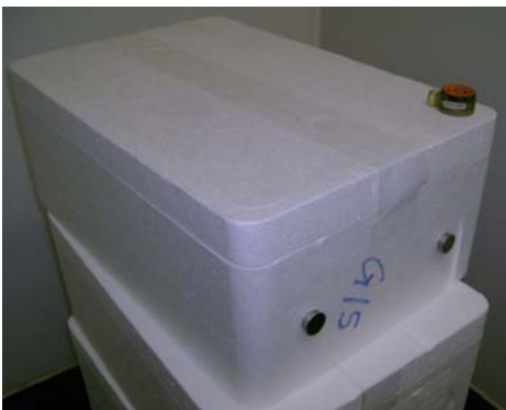
Figure 34. EPS boxes, Onset Tidbit and DS1922L ibutton temperature data loggers on outer surface.
